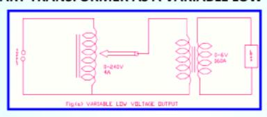
The above connection diagram shows that the 4A, 240 Volt Dimmer is connected with a 40:1 step down transformer just to provide a variable voltage output at 160 amps rated current. As well as with the same procedure we may use the higher rating Dimmer for different purposes. This being the most useable common circuit for High Current D.C Power Supplies as Stator Heating Rectiformers, Electroplating Sets and etc.
