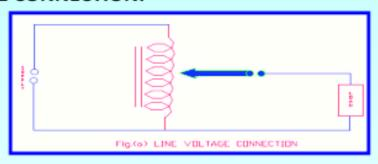
The input voltage (0-240 v) is applied across the whole winding and the output. Voltage is variable from zero up to the input voltage. Rated current can be drawn at or near about full output. For a constant impedance load which draws maximum current at the Dimmer rated input voltage can be controlled from zero to the line voltage. The connection diagram the above mentioned is the most COMMONLY USED circuit for all GENERAL PURPOSE-VOLTAGE-CURRENTLIGHT-SPEED-HEAT CONTROL & etc.
